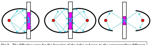
Fig.2 The Effective zone for the focusing of the infra red rays in the corresponding different mirror systems. The length of this zone in the four mirror furnace is much shorter than that of both the single and the double mirror system.
