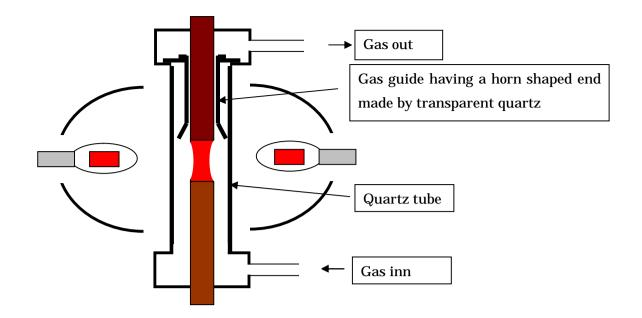
Fig.5 Schematic diagram of the gas guide having a horn shaped end inserted into the quartz tube.
