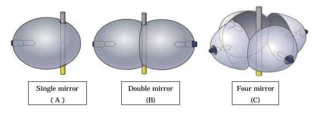
Fig.1 Three types of the focusing system for the optical floating zone furnace. In the case of the four mirror system, the center portion of the mirror system has wide space and both the single and the double mirror system has no such space between the quartz tube and the mirrors. This meant that the four mirror system could prevent the deposition of small particles from the surface of the quartz tube (Fig. 2).
