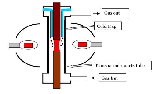
Fig.4 Schematic diagram of the cold trap inserted in the quartz tube and focusing scheme. Small particles from the molten zone would be condensed on the cold trap rather than the surface of the quartz tube, then can keep its clean condition more long time compared to the normal case without the cold trap.
